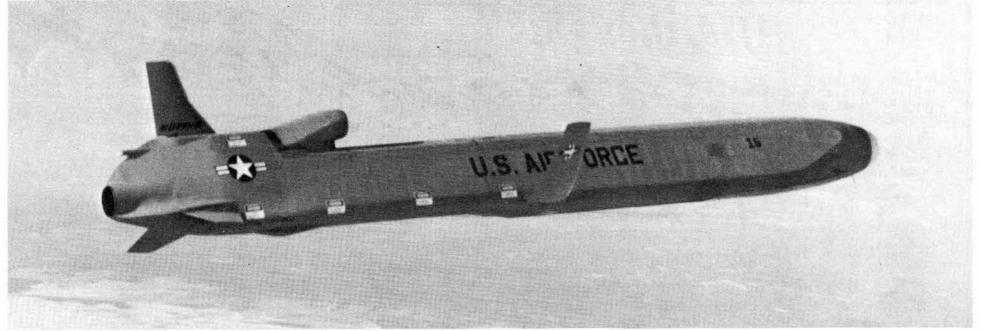
CARRYING A SANDIA W80 WARHEAD, the Boeing Air Launched Cruise Missile is scheduled for first alert capability in the fall of 1981. Production W80
